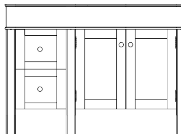
City full depth vanity unit 3 door with integral 2 drawer stack in lieu of door.
