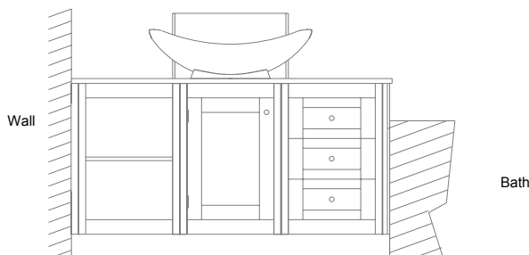
Showing special configuration of units between wall and bath.
